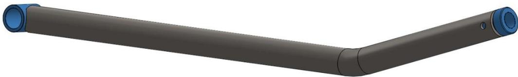
3. Notch the long leg of the 2" x .25" DOM tubes for the Bushed DOM. This is where you can set the angle of your bushing in the trailing arm. You can also set the bushings at 0\* and build the angle in to your chassis mounting brackets. Once angle is set, fully weld the Bushed DOM in place. Do not weld with poly bushings installed. If the Bushed DOM needs to be assembled for your welding, check out our Bushed DOM Mock Up Pucks (P/N: R2019)
